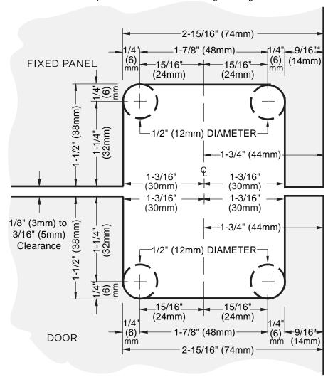
\* The 9/16" (14mm) measurement is ok as long as the fixed panel side clearance is the same as the door side clearance. If not, make the appropriate add-on or deduction.
