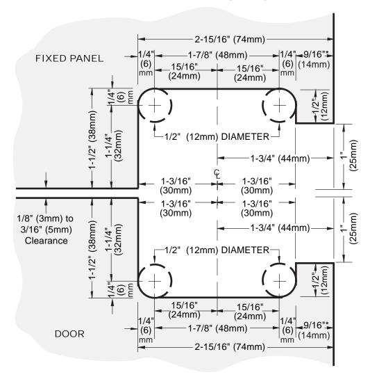
\* The 9/16" (14mm) measurement is ok as long as the fixed panel side clearance is the same as the door side clearance. If not, make the appropriate add-on or deduction.
